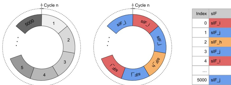
Again, while this figure aims to visualize the concept for 3 sIF (here red, blue and yellow), the NEV chip can support up to 4096 sIF.
