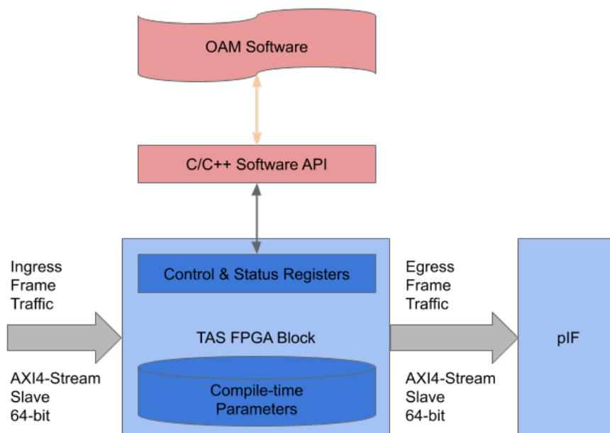
Via a software API, bandwidth, traffic priority, traffic burstiness, etc. can be controlled by assigning certain Service Interfaces to timeslots in the Traffic Shaper. Short cycle times, enabled by network protocol processing in PL, keep processing latencies short and deterministic.
