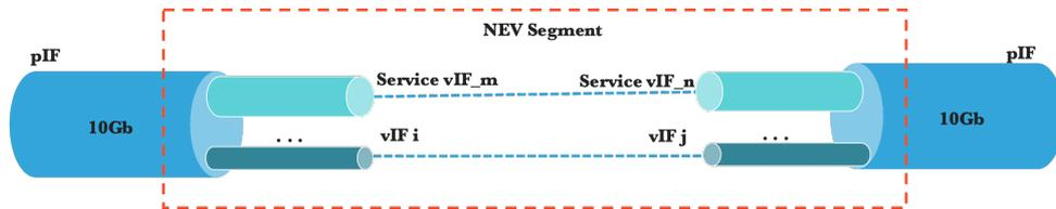
As a result, a physical network interface (pIF) can carry many NEV Service Virtual Interfaces (sIF). Algotblu developed a centralized PTS (Primary Telco Services) OAM system to control and manage this virtualization, including dynamic adjustments of bandwidth, on a network segment by network segment basis.
