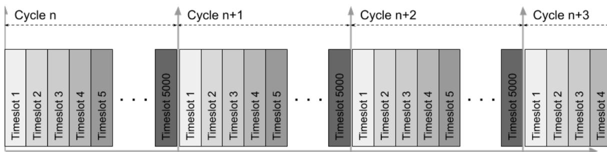
Another way to represent this can be a “wheel” with 5000 Timeslots where each sIF can occupy zero, or more, Timeslots. The following figure visualizes how different sIF can run using NEV.
